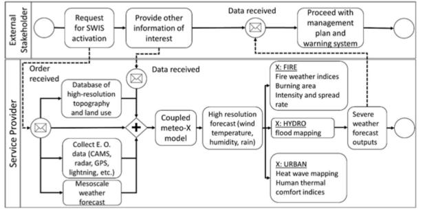
Figure 10. Severe weather integrated system, Greece
