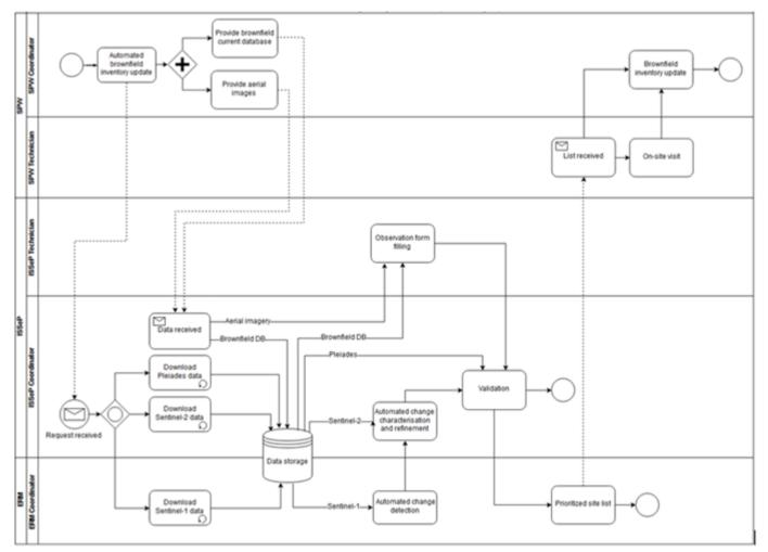
Figure 14. Automated brownfield monitoring using SAR and optical imagery
